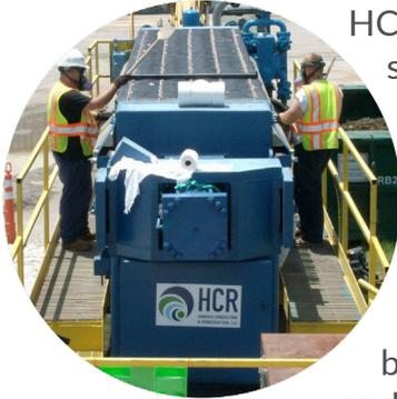
HCR comprehensive sludge dewatering technologies reduce volumes of liquid/solid mixtures by up to 80%. The end result is a reduction in transportation and disposal costs, and a step towards compliance with the EPA regulations to minimize waste generation. HCR dewatering options include High Pressure Plate and Frame Filter pressing, Belt Press filtering, Centrifuge processing and Geomembrane solutions.
