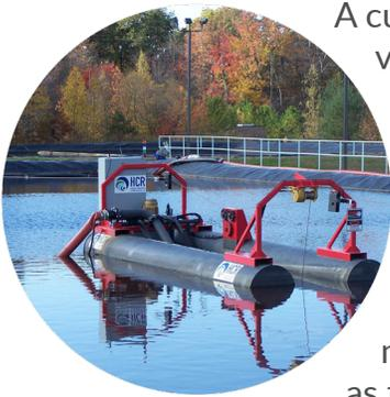
A cutter-head dredge enables the removal of sludge and sediment at a fixed or variable depth over the surface area of a lagoon.
