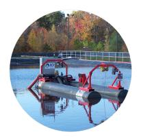
A cutter-head dredge enables the removal of sludge and sediment at a fixed or variable depth over the surface area of a lagoon. The dredge is used on basins where the agitation of the sludge and sediments is necessary to achieve effective removal, and where there is an adequate layer of surface water to float the dredge.
